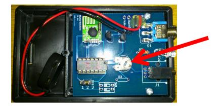
We suggest adjusting by depressing LC button and turn the potentiometer very slowly until the car creeps and then just a little back until it stops, this should give the optimal adjustments.
